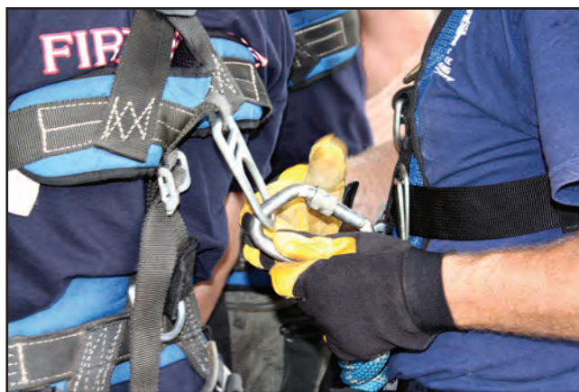
Figure 5.5 Equipment that must be checked before entering a rescue environment includes safety line connections.
