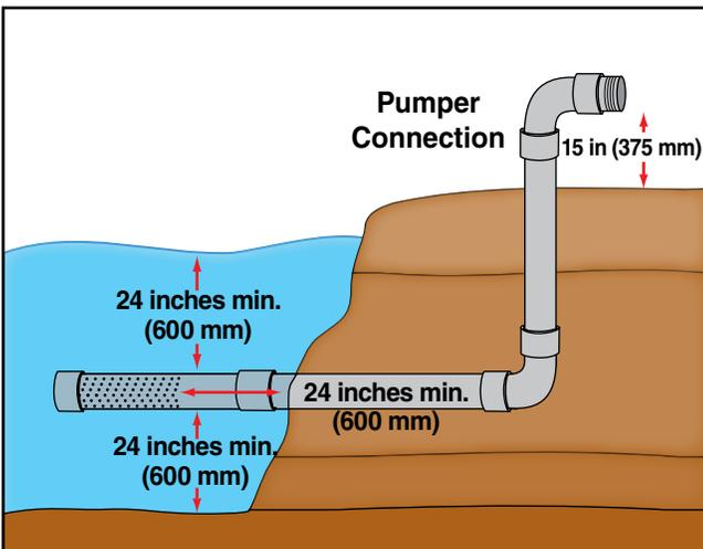
**Figure 4.8** A dry hydrant installation.
