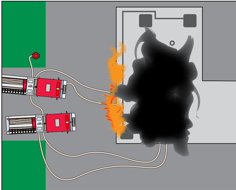
**Figure 4.12** Dual pumping operations.
