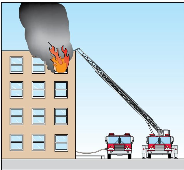
**Figure 4.6a** The aerial is positioned outside the pumper because the building is less than five stories tall.
