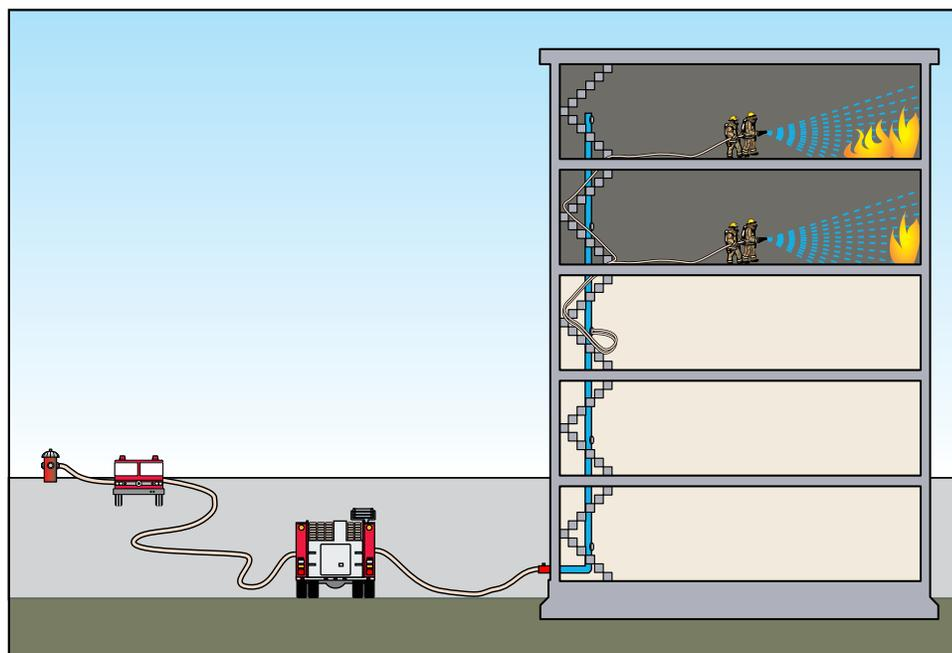
**Figure 4.13** Tandem pumping operations.
