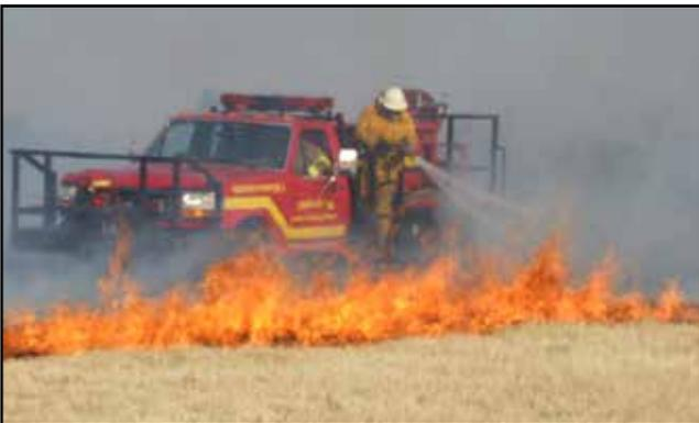
**Figure 4.14** A wildland fire apparatus using pump and roll attack operations.
