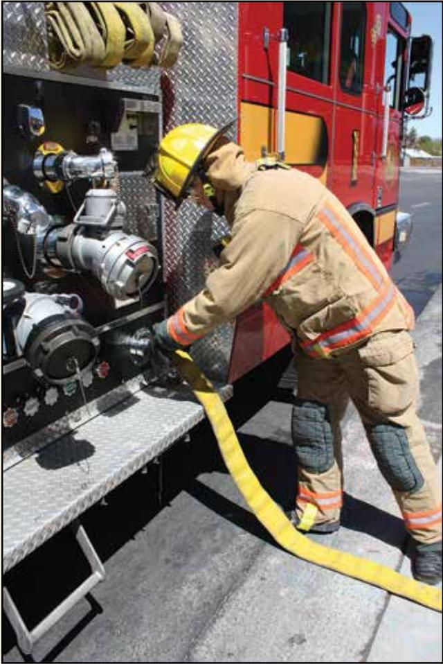
**Step 5:** Connect 2½- or 3-inch (65 or 77 mm) hoselines to the apparatus intake.
