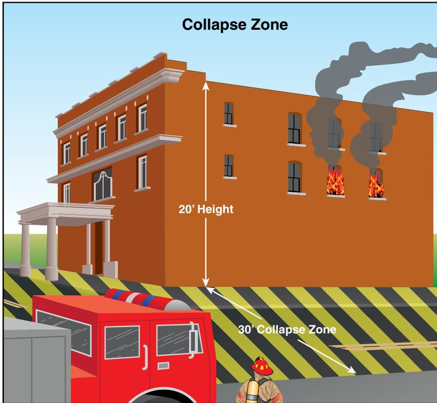
**Figure 4.4** Position the apparatus outside of the collapse zone.
