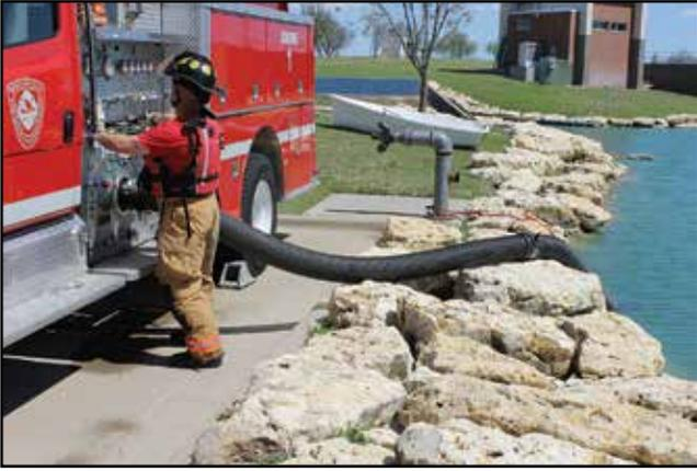
**Figure 4.7** A pumping apparatus set up for a drafting operation from a static water supply.
