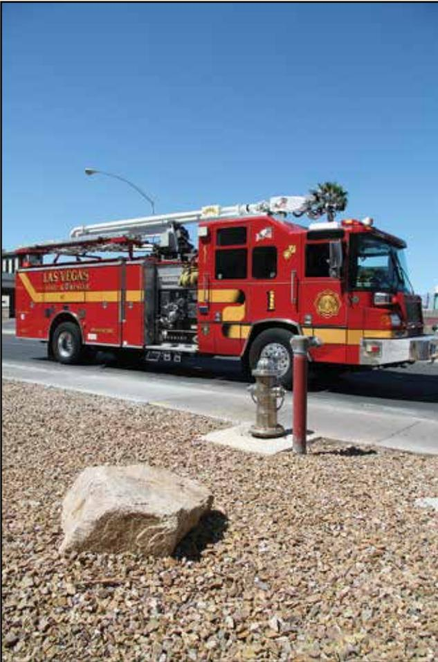
**Step 1:** Position apparatus a few feet (meters) short of hydrant. Chock wheels.
