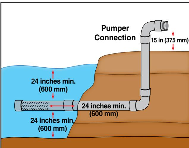
**Figure 4.8** A dry hydrant installation.
