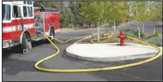
**Figure 4.11** An apparatus connected to a hydrant using two 2½ inch (65 mm) hoselines.
