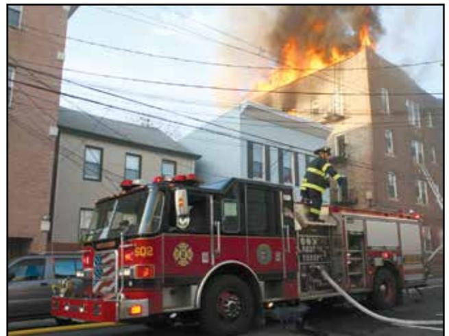
**Figure 4.5** Parking a pumper directly below a large number of utility lines may be dangerous, especially if fire or weather conditions cause them to fall. *Courtesy of Ron Jeffers.*
