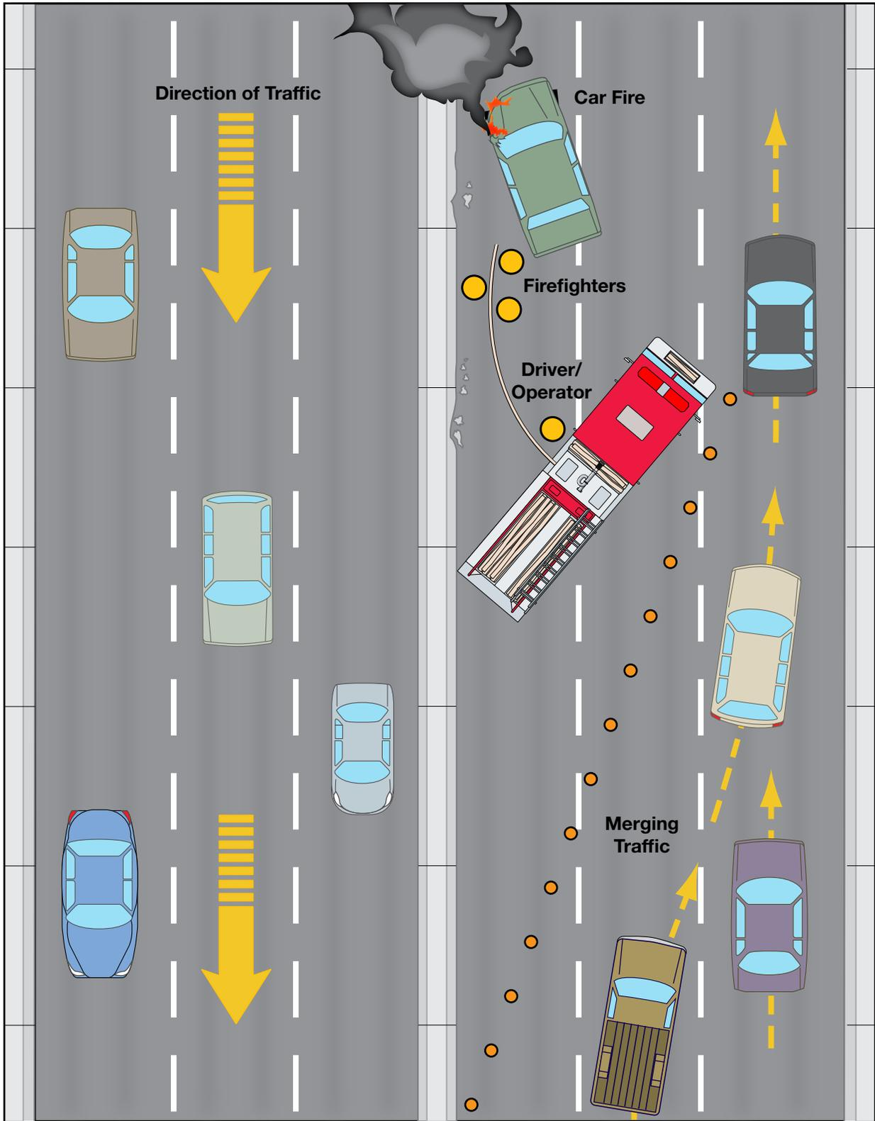
**Figure 4.19** The placement of the apparatus shields the firefighters from oncoming traffic.
