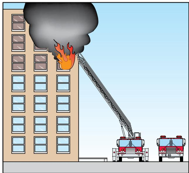
**Figure 4.6b** The aerial is positioned inside the pumper because the building is more than five stories tall.
