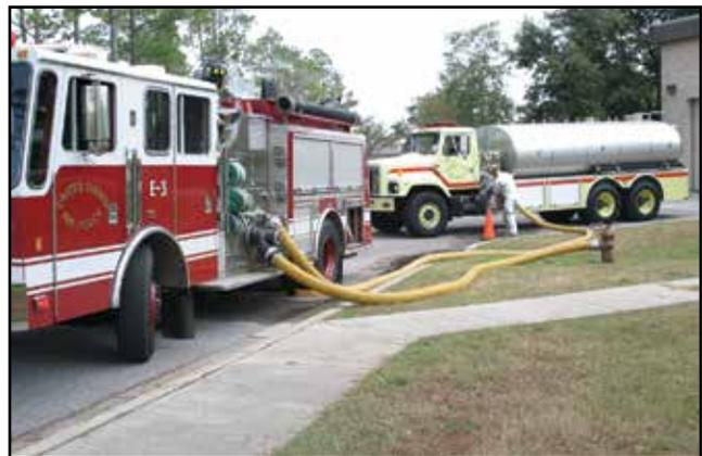
**Figure 4.3** Lay supply hose to the side of the street from hydrant to pumper.
