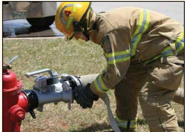
**Step 5:** Connect additional 2½- or 3-inch (65 or 77 mm) lines to gate valve and apparatus.
