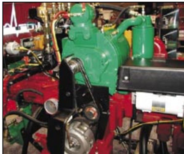
*This is a Waterous compressed air foam system. Note the green air compressor and the attached drive belt mounted above the red fire pump.*
