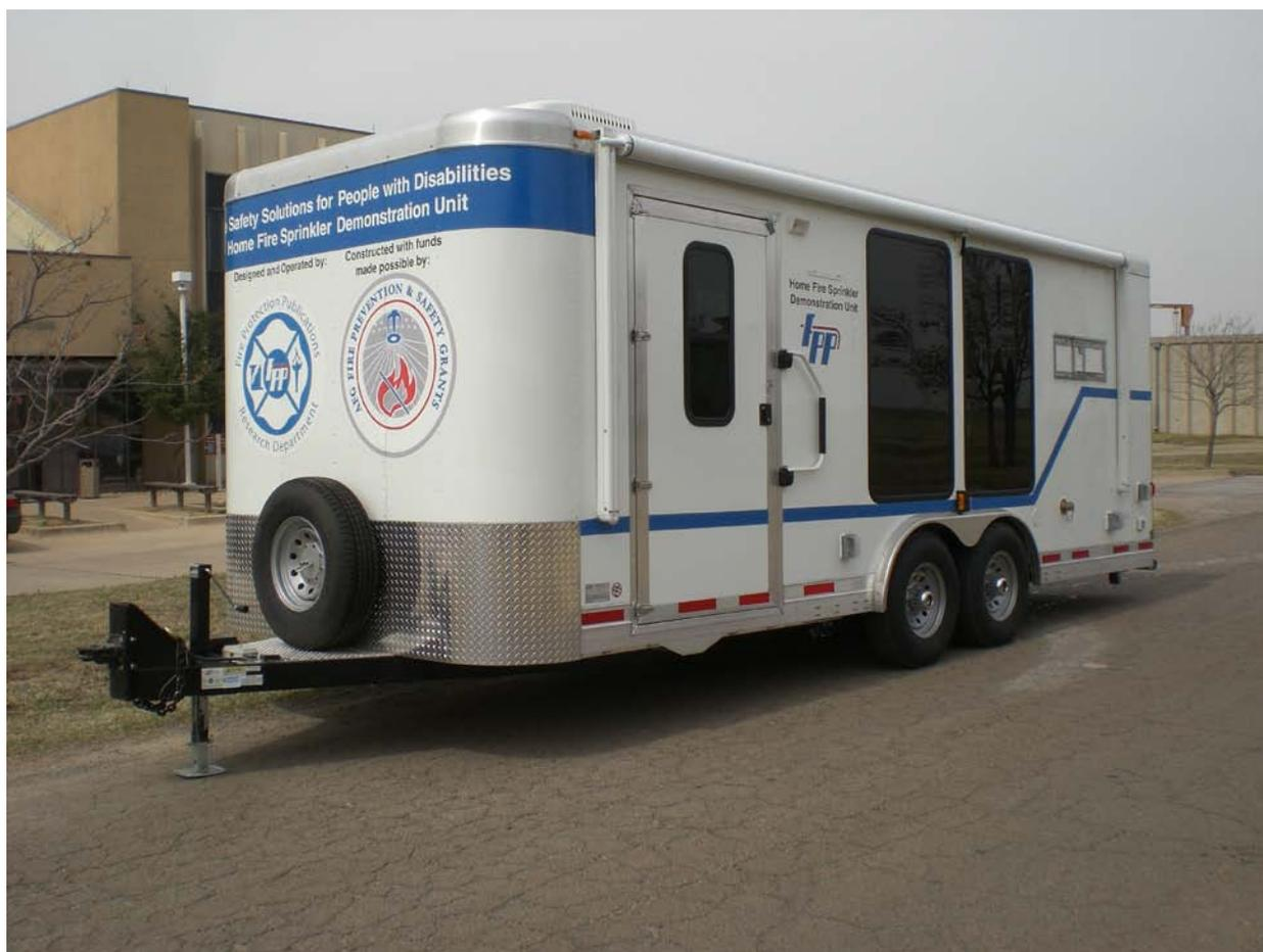
The design of the trailer consists of three rooms: An interior viewing room, a live fire demonstration (middle) room, and the sprinkler control room. The demonstrations may be viewed from the interior which is climate controlled, or externally from either side through large, low windows. The trailer has an ADA compliant ramp to bring people into the interior viewing room and a large retractable awning on the outside for shade when needed.
