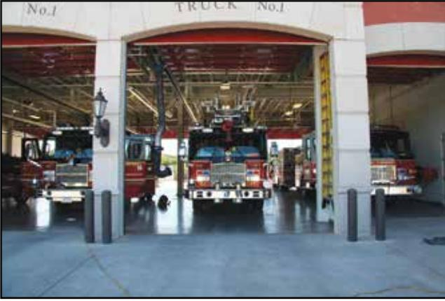
**Figure 10.12** Fire stations with drive-through bays all but eliminate the possibility of accidents that occur when apparatus are backed into stations.
