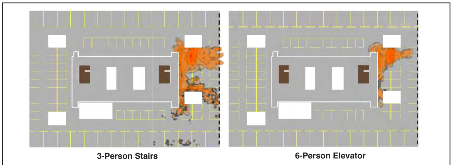
Figure 91: Visualization of HRR for a medium growth fire for a 3-person crew using the stairs (left) and a 6-person crew using the elevators (right) at the time firefighters make entry to the floor
