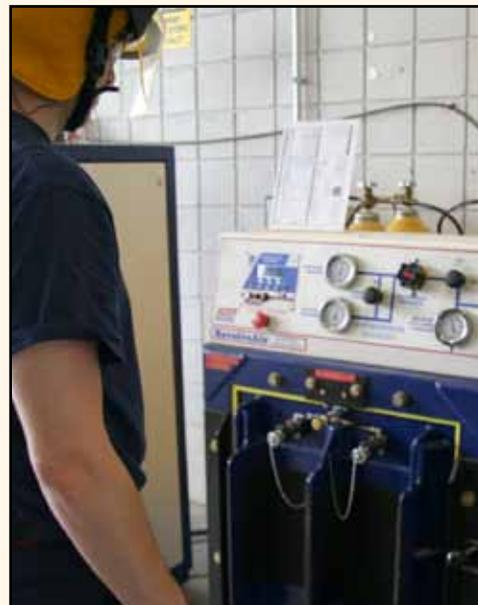
**Step 7:** Set the cylinder pressure adjustment on the compressor (if applicable) or manifold to the desired full-cylinder pressure. If there is no cylinder pressure adjustment, watch the pressure gauge on the cylinder during filling to determine when it is full.
