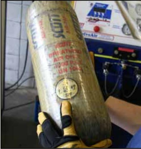
**Step 1:** Check the hydrostatic test date of the cylinder.
