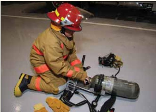
**Step 11:** If air leaks are detected, determine if connections need to be tightened or if valves, donning switch, etc. need to be adjusted. Otherwise SCBA with audible leaks due to malfunctions shall be removed from service, tagged, and reported to the officer.
