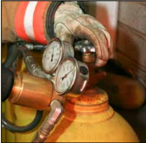
**Step 8:** Close the cascade cylinder valve when the pressures of the SCBA and the cascade cylinder equalize.
