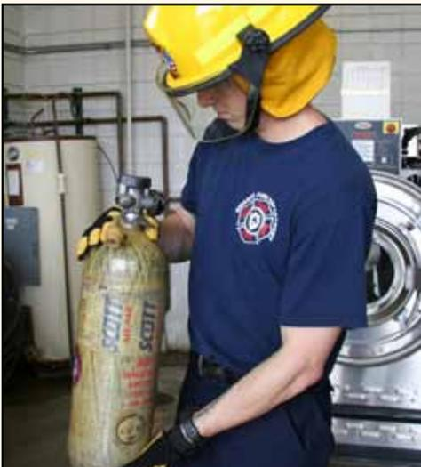
**Step 2:** Inspect the SCBA cylinder for damage such as deep nicks, cuts, gouges, or discoloration from heat. If the cylinder is damaged or out of hydrostatic test date, remove it from service and tag it for further inspection and hydrostatic testing.
