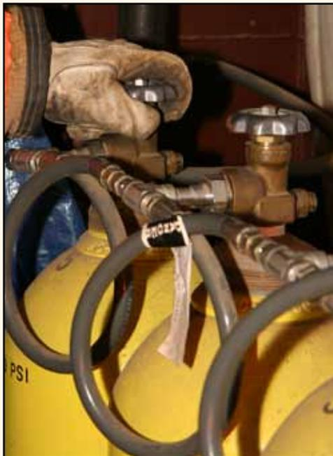
**Step 9:** Close the valve or valves at the cascade system manifold and/or fill line if the system is so equipped.
