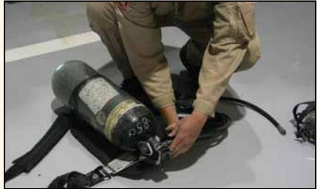
**Step 7:** Check that gauges and/or indicators (i.e. heads-up display) are providing similar pressure readings. Manufacturers' guidelines determine the acceptable range.
