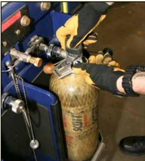
**Step 10:** Close the fill station valve when the cylinder is full.
