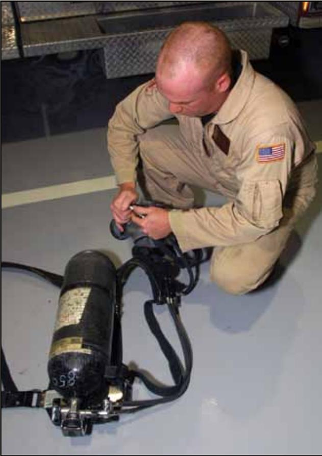
**Step 1:** Identify all components of SCBA are present: harness assembly, cylinder, facepiece, and PASS device.
