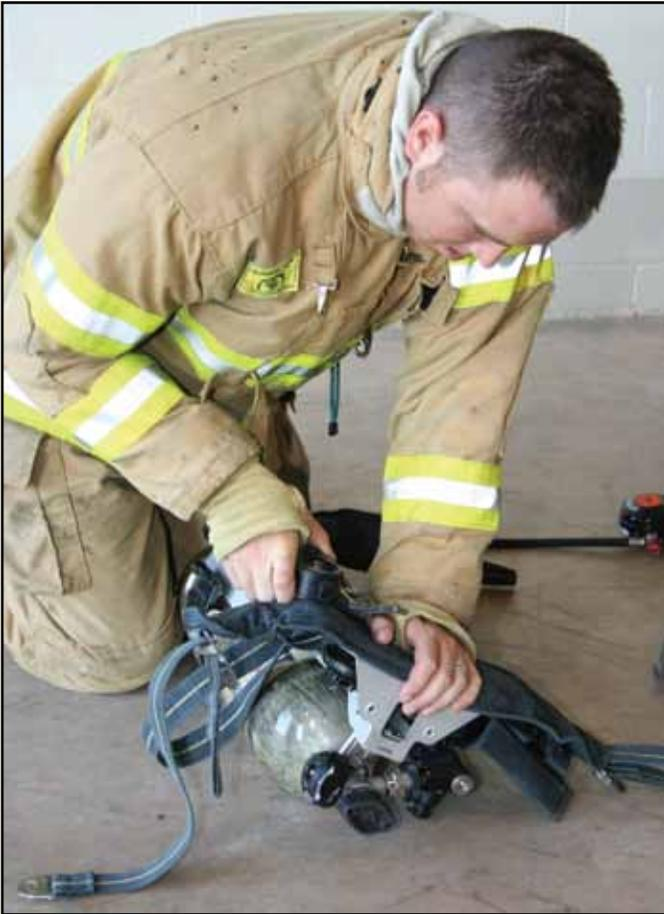
**Step 1:** Position the SCBA with the valve end of the cylinder away from the body, the cylinder down, and back frame up. All harness straps are fully extended and untangled.
