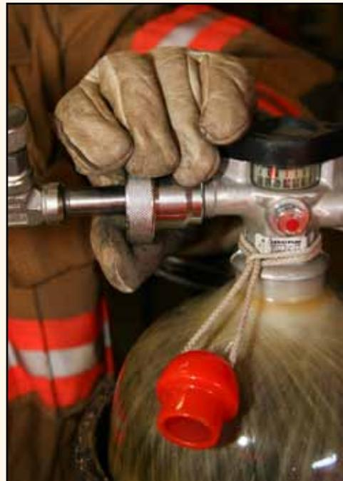
**Step 12:** Disconnect the fill hose from the SCBA cylinder.
