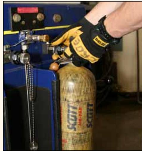
**Step 13:** Disconnect the fill hose from the SCBA cylinder.
