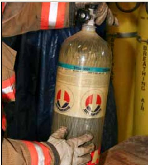
**Step 2:** Inspect the SCBA cylinder for damage such as deep nicks, cuts, gouges, or discoloration from heat. If the cylinder is damaged or is out of hydrostatic test date, remove it from service and tag it for further inspection and hydrostatic testing.
