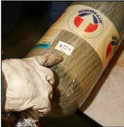
**Step 1:** Check the hydrostatic test date and recommended fill pressure of the cylinder.
