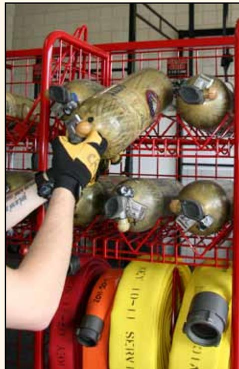
**Step 14:** Remove the SCBA cylinder from the fill station and return the cylinder to proper storage.
