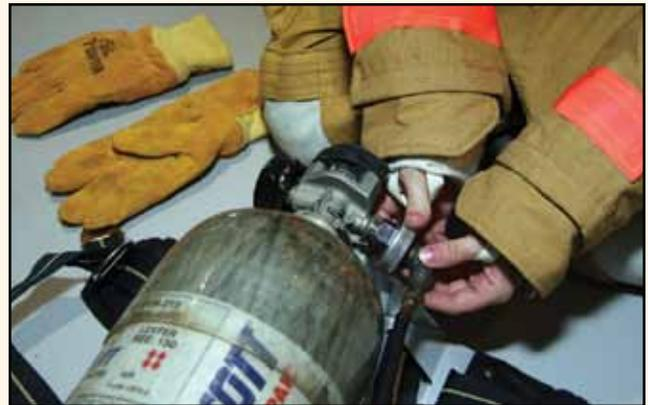
**Step 13:** Check pressure reading on remote gauge and/or indicators and report reading.
