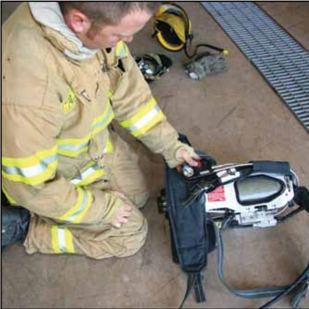
**Step 1:** Position SCBA with the valve end of the cylinder toward the body, the cylinder down, and back frame up. All harness straps are fully extended and untangled.
