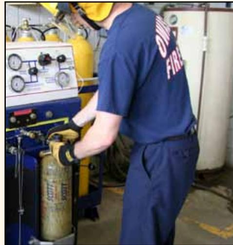
**Step 4:** Connect the fill hose to the cylinder and close bleed valve on fill hose.
