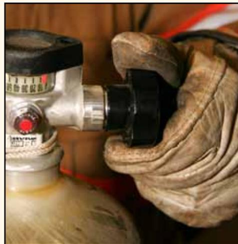
**Step 7:** Open the valve of the cascade cylinder that has the least pressure but that has more pressure than the SCBA cylinder.
