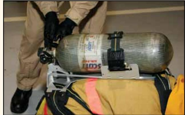
**Step 11:** Slowly open the cylinder valve fully and listen for an audible alarm and leaks as the system pressurizes.
