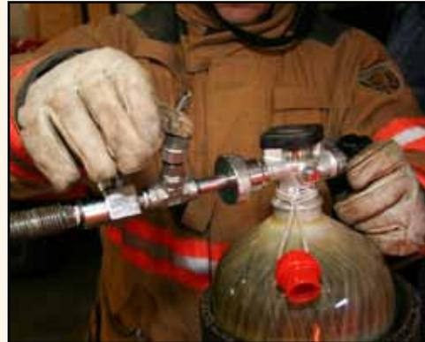
**Step 11:** Open the hose bleed valve to bleed off excess pressure between the cylinder valve and the valve on the fill hose.
