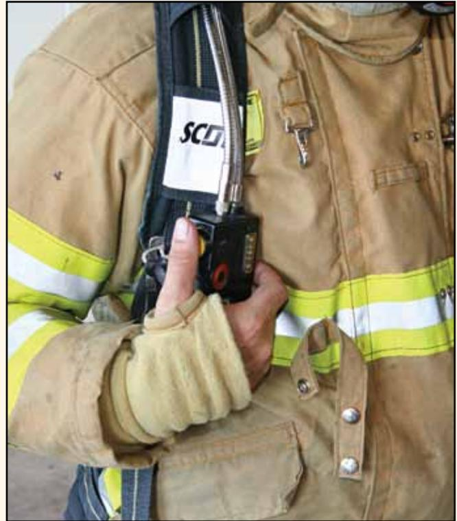
**Step 11:** Activate external PASS device, if not equipped with integrated device.
